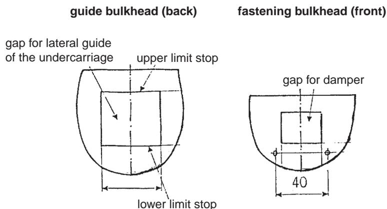
Fix the lower limit stop in such a way that the retractable undercarriage rests with an initial stress of 1-2 mm. The lateral guide should not have more than 0.5 mm of positive allowance. We recommend to screw plastic ledges onto the bulkhead for the lateral guide that can then be adjusted very precisely. Grease the guide a bit to obtain a safe functioning.
