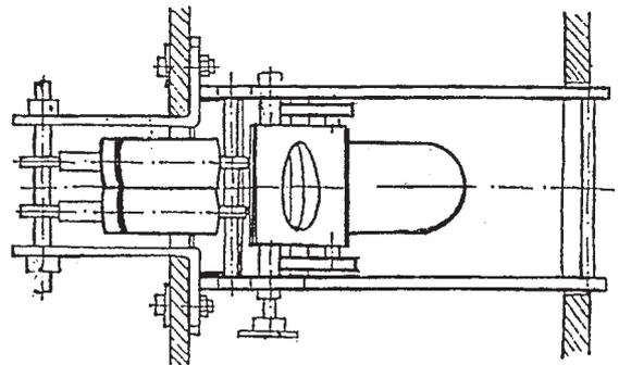
For very rough flight practice we recommend mounting the thrust bearing according to figure III. This fastening method relieves the fastening bulkhead as the forces are lead directly to the fuselage. The additional longitudinal bulkheads and the transverse bulkhead give the undercarriage an optimal support.
